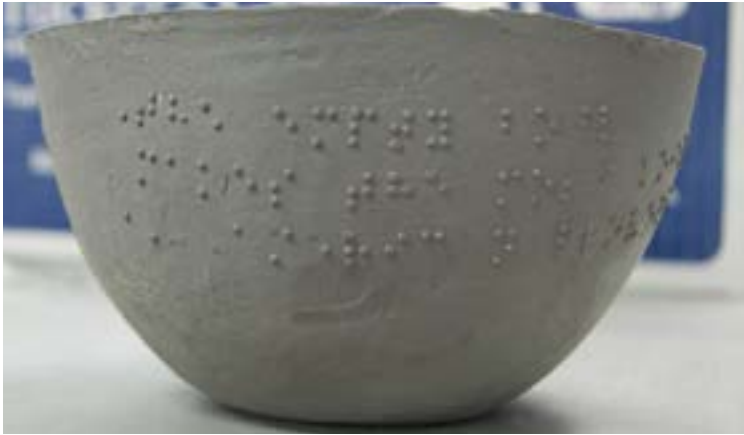
Figure 16. A cast made by a mould without the bowl's curvature taken into account
