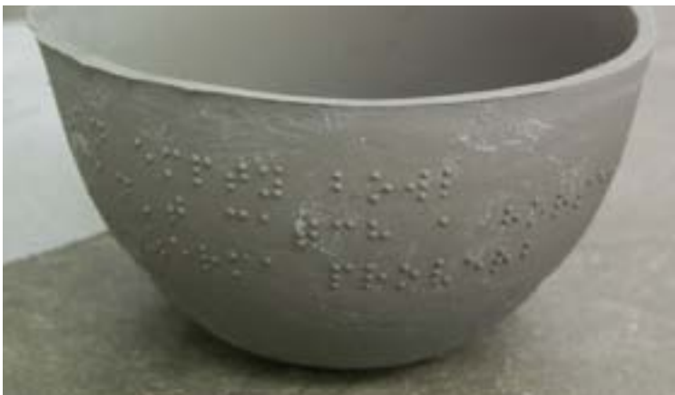
Figure 17. A cast made by a mould with the bowl's curvature taken into account
